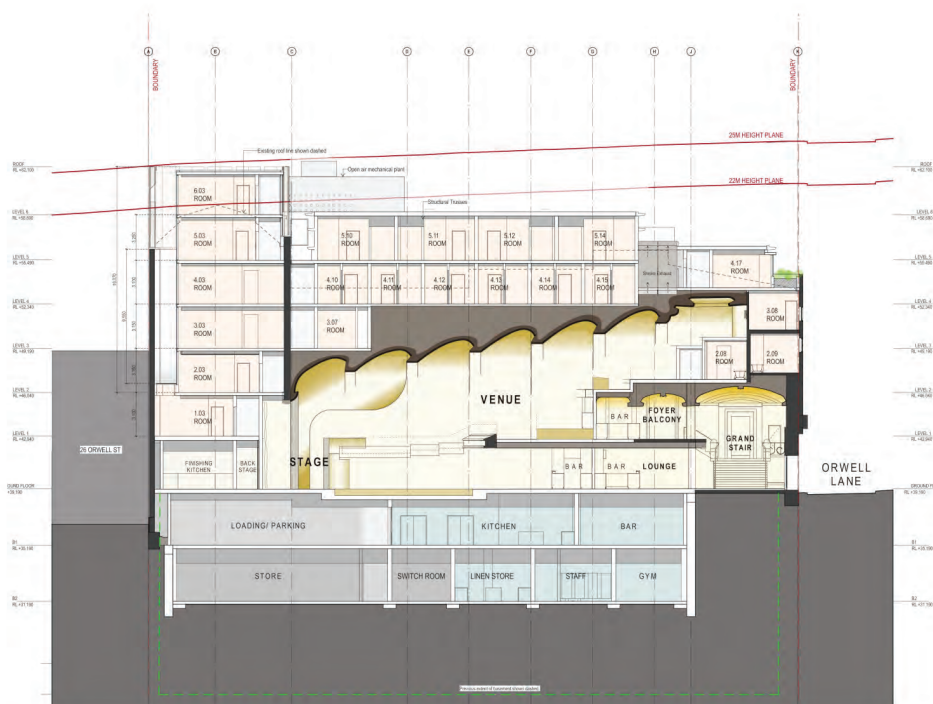
Figure 6: Cross Section, indicating height locations for the various levels of the existing and proposed building.
